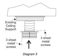
The connection between the appliance and the Retro Connector may be completed with sections of black direct vent pipe, together with an adjustable length.
